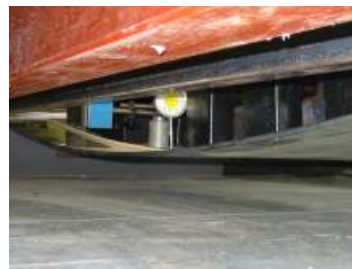
Testing the Glass Deviation
