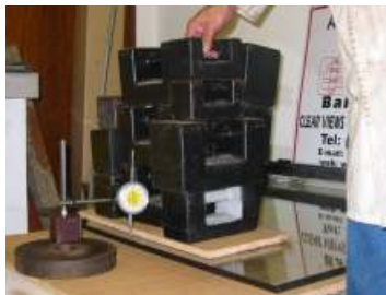
SABS Testing on Balustrade Glass
