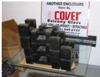
SABS Testing on Balustrade Glass
